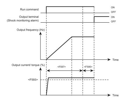
\* When under setting time of <F595>, and the inverter is in acceleration/ deceleration status or overcurrent stall during detection activates, detection time will be reset.
