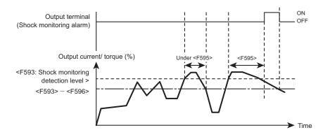
When setting <F591>="1", the inverter trips after overcurrent/ overtorque is detected for the period of time set with <F595: Shock monitoring detection time >. The alarm signal remains ON after trip "OtC3".
