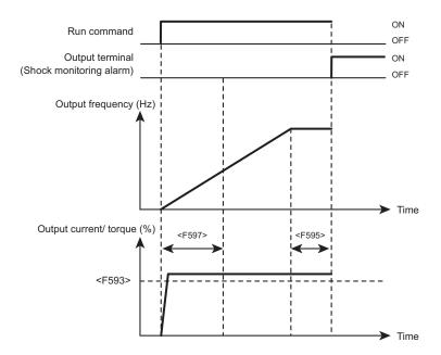
\* When under setting time of <F595>, and the inverter is in acceleration/ deceleration status or overcurrent stall during detection activates, detection time will be reset.
