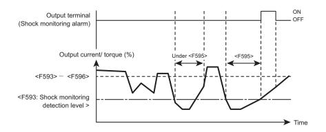
When setting <F591>="1", the inverter trips after undercurrent/ undertorque is detected for the period of time set with <F595: Shock monitoring detection time >. The alarm signal remains ON after trip"OtC3".
